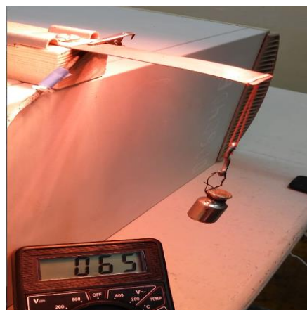
Figure 2. Restoration of deformation of the plate under the counteracting load during heating
